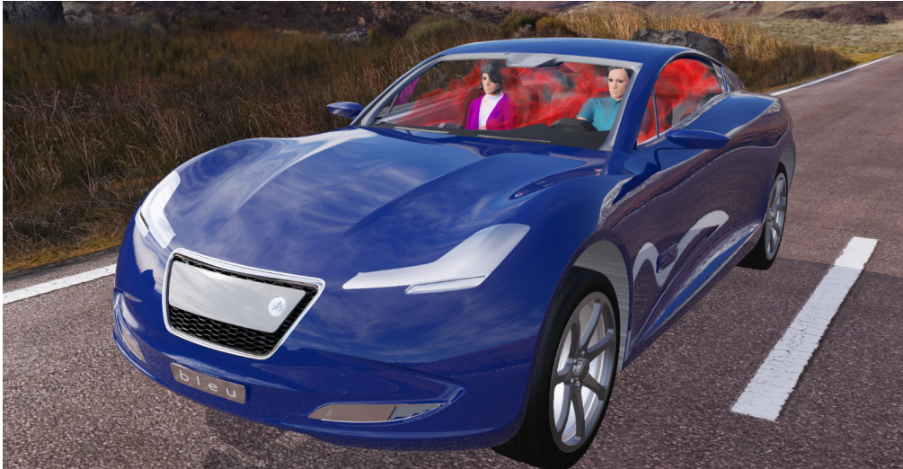
Cooldown prediction of flow & temperature distribution inside a cabin with multiple humans
